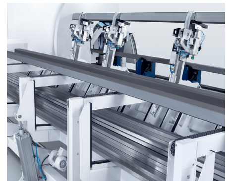
The swivel-mounted conveyor system can be used for small lot sizes and custom profiles.
